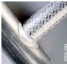
The COMPOTIG function combines the beneficial qualities of both direct and alternating current. It simplifies joining aluminium alloys and decreases the number of defects.
