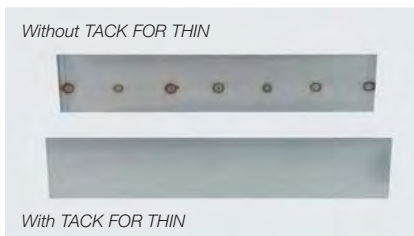
The difference in the tack welds is clearly visible. TACK FOR THIN was used to weld the piece on the bottom, and regular TIG was used on the piece on the top.
