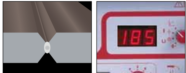
Penetration pass Short-Arc MIG, thickness < 25 mm.
