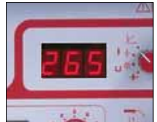
Spray-Arc MIG, thickness < 10 mm.
