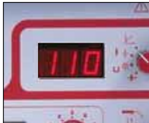
Short-Arc MIG, thickness < 3.0 mm.
