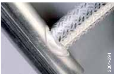
The COMPOTIG function combines the beneficial qualities of both direct and alternating current. It simplifies joining aluminium alloys and decreases the number of defects.
