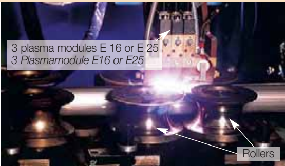
Fig.6: Integration of the tricathode between the forming rolls
